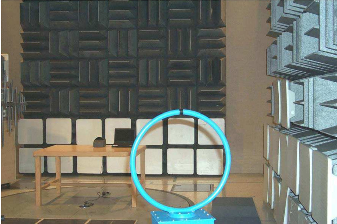
Model AT9000 Full Page Reader Carrier Frequency / Emissions Bandwidth / Spurious Emissions 9KHz to 30 MHz
