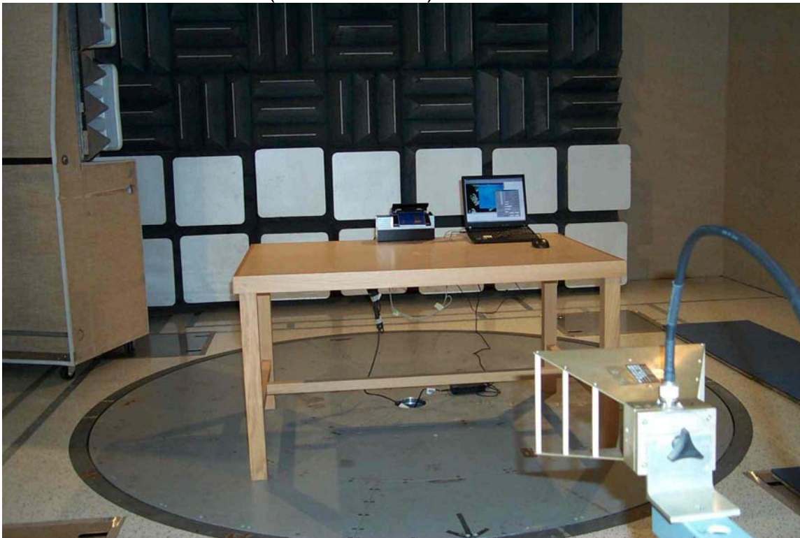
PV33 Radiated Emissions (1 GHz – 5 GHz)
