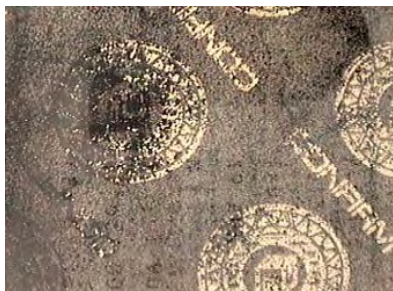
Figure 5: Damaged 3M™ Confirm™ Laminate
