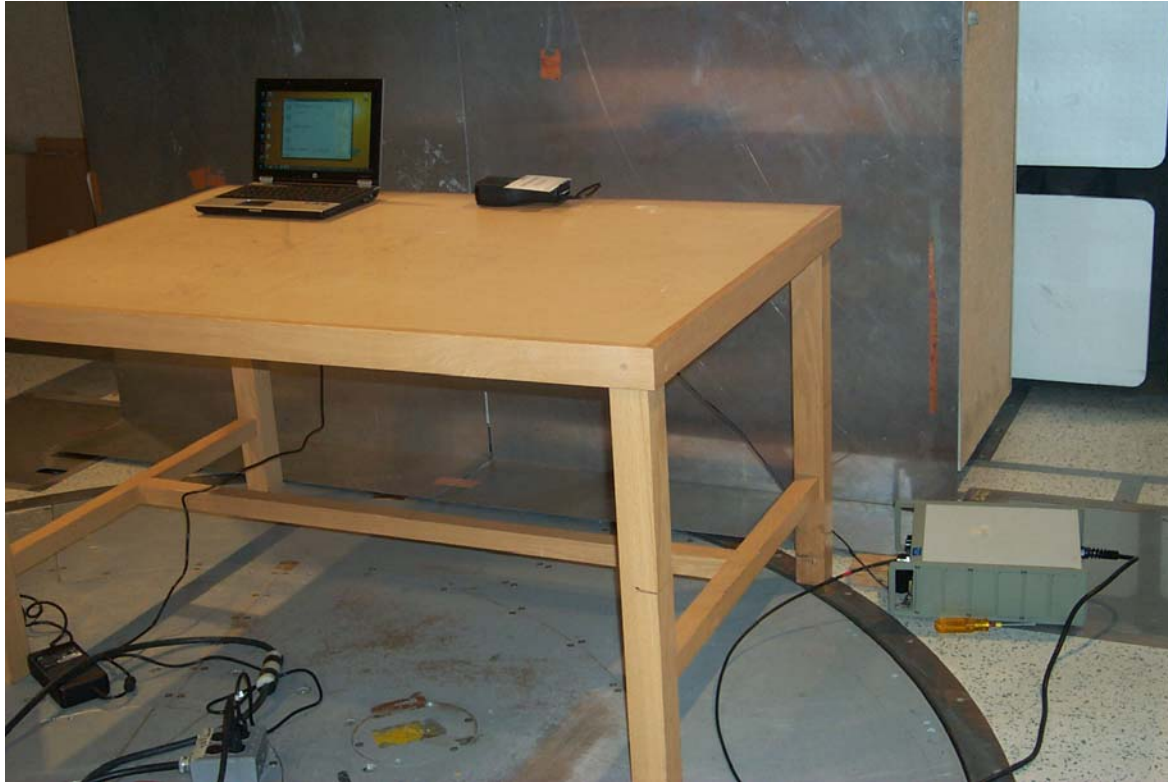
Conducted Emissions (with charger)
