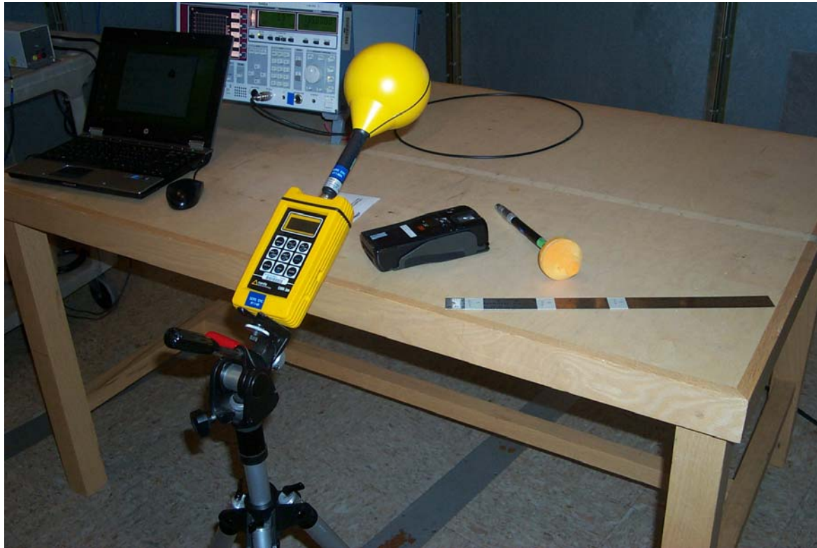
RF Exposure Measurement
