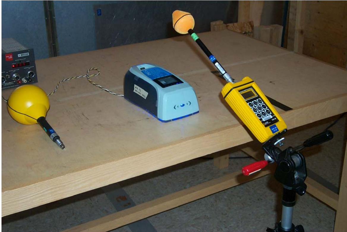
RF Exposure Measurement E-Field and H-Field
