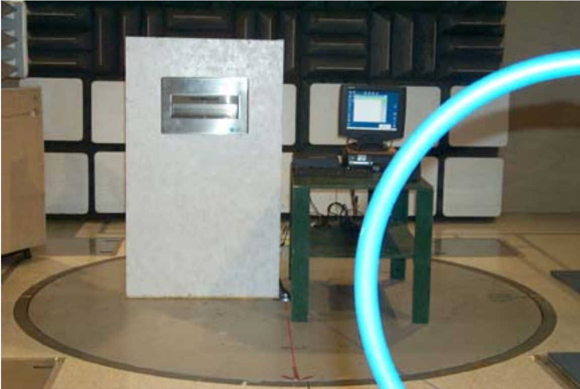
TEST SETUP Spurious Emissions 12 to 30 MHz
