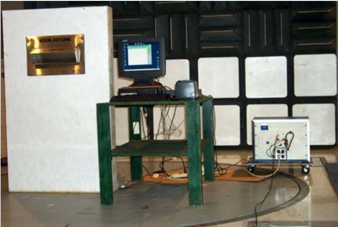
TEST SETUP Conducted Emissions
