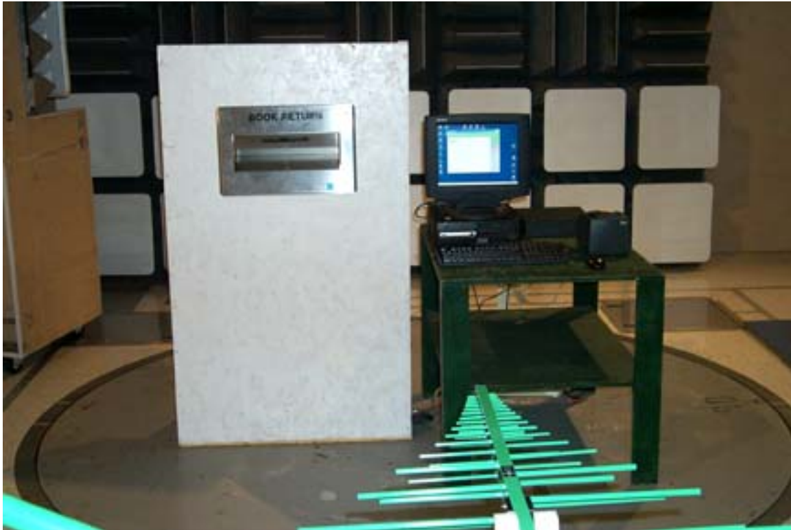
TEST SETUP Radiated and Spurious Emissions 30 to 1000 MHz
