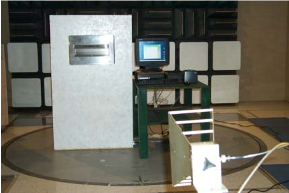
TEST SETUP Radiated Emissions 1 to 10 GHz
