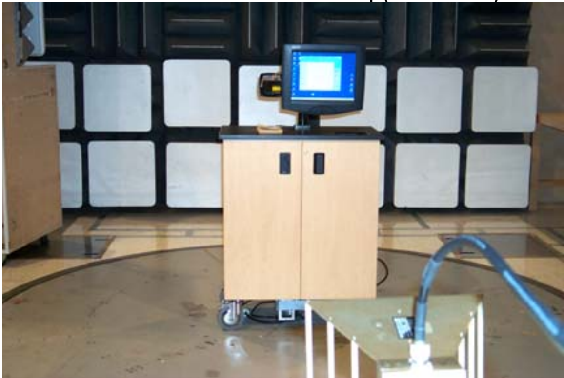
Model 812 Radiated Emissions Test Setup (1 GHz – 5 GHz)
