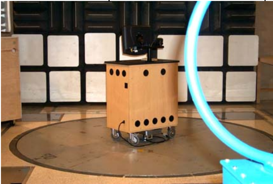
Emissions Bandwidth and Spurious Emissions below 30 MHz Test Setup
