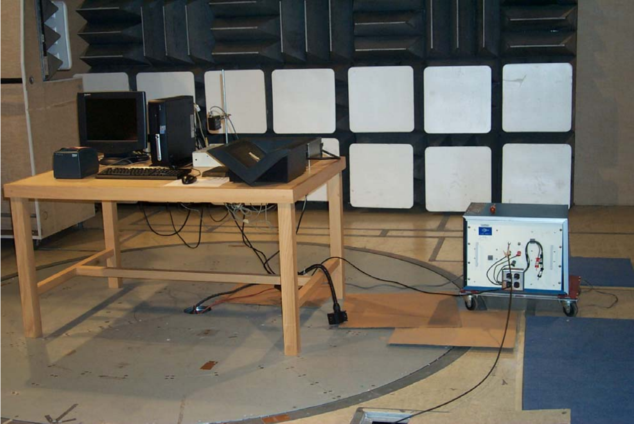
Conducted Emissions Test Setup Photo:
