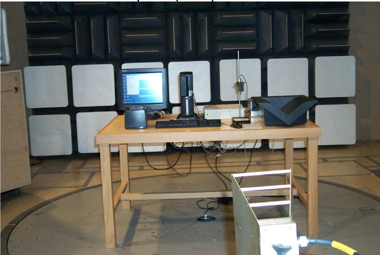
Radiated Emissions Test Setup Photo (1-5GHz):
