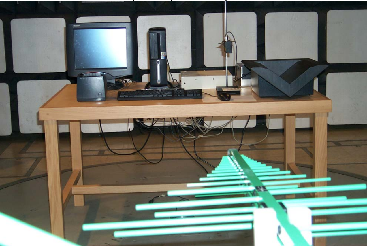
Radiated Emissions Test Setup Photo (30-1000MHz):
