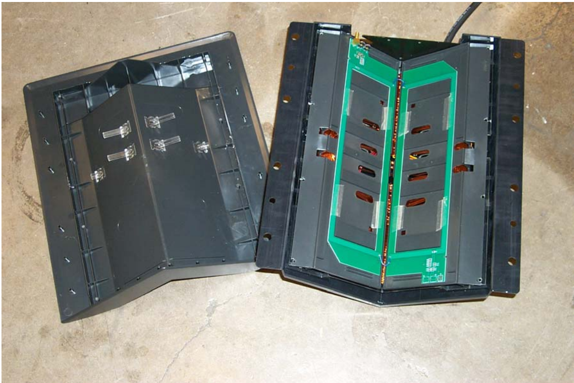
Antenna Location in V-Box
