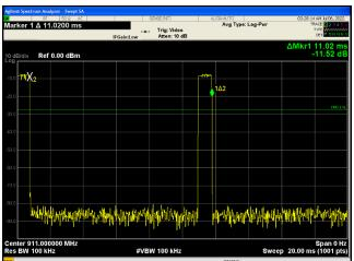
The total number of pulses over 100 ms/11 ms = 9Transmission On time per burst = 0.820 msTotal on time over  $100 \text{ ms} = 0.820 \text{ms} \times 9 = 7.5 \text{ms}$ Duty Cycle Correction Factor =  $20 \log (7.5 \text{ms}/100 \text{ms}) = -22.6 \text{dB}$
