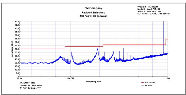
FCC Part 15.209 Radiated Emissions in restricted band - Low Channel
