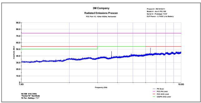
FCC Part 15.209 Radiated Emissions in restricted band - High Channel
