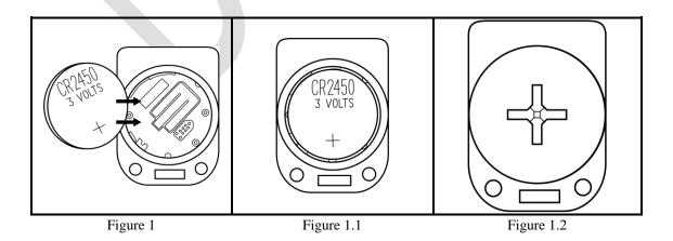
**NOTE:** To maintain the safety of the device, it is recommended to replace the battery with a UL or ETL marked / listed CR2450 Lithium Manganese Dioxide coin cell battery.
