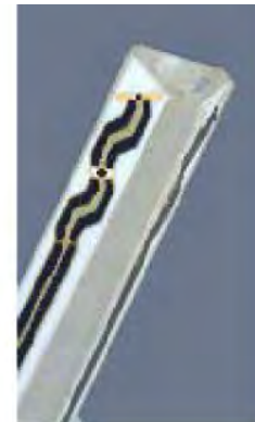
Figure 2.3 Probe Thick-Film Technique
