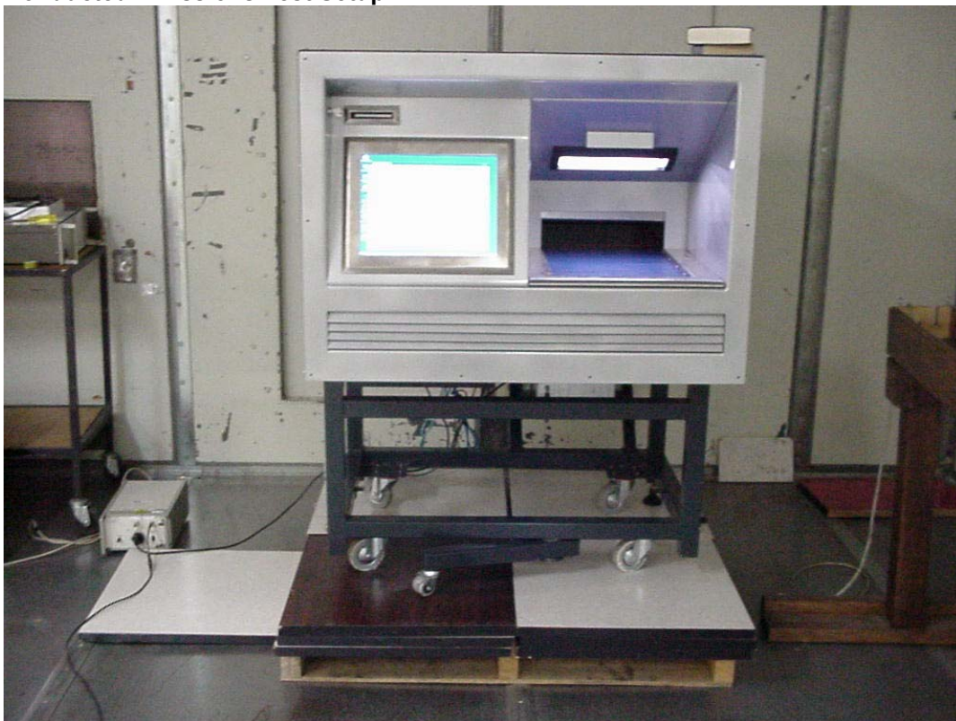
Conducted Emissions Test Setup
