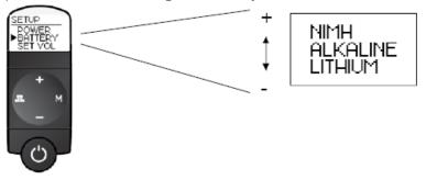
**To specify the preset (default) volume level:** Select the "SET VOL" option in the Setup menu. Press and release the (M) button to select the current volume level as default. The factory default is level 3.
