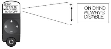
**To select Auto Off power management:** Select the "AUTO OFF" option in the Setup menu. Use the (-) and (+) buttons to scroll through the list of options. Press and release the (M) button to select. The factory default is "ENABLE".
