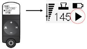
2. End playback: Depress and release the (M) button. The stethoscope will stop playing the sound track and will return to its previous operational mode.
