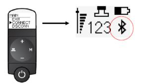
A Bluetooth connection with the stethoscope will automatically be ended if no data transfers occur in a 90 second period. Alternatively, they can be manually ended using the "DISCONN" (disconnect) option of the Main menu.
