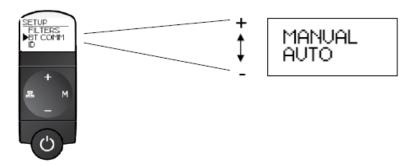
**To obtain model and software version information**: Select the "ID" option in the Setup menu. Use the (-) and (+) buttons to scroll through the list of reference numbers. Press "M" to return to the operating mode of the stethoscope.
