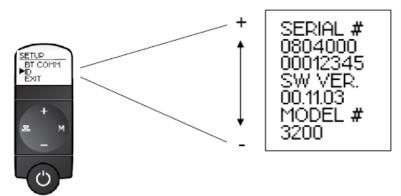
To leave the Setup menu: Use the (M) button to select the "EXIT" entry and return to the operating mode of the stethoscope.
