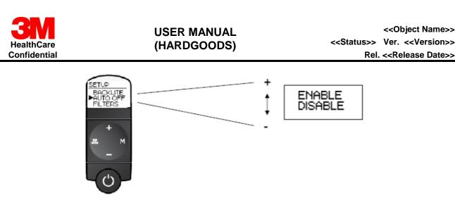
The Auto On feature powers on the stethoscope from its standby mode when contact is detected with the diaphragm. With the Auto Off feature, power is turned off when user activity is no longer detected (the stethoscope returns to its standby mode after a delay equal to the Power On time.)
