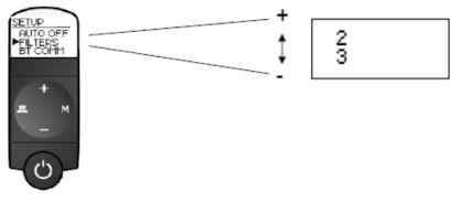
**To specify Bluetooth mode:** Select the "BT COMM" option in the Setup menu. Use the (-) and (+) buttons to scroll through the list of options. The MANUAL option means that the Bluetooth link can be used for data transfers but requires user activation. The AUTO option means that the Bluetooth link is powered whenever the stethoscope is in an active mode. Press and release the (M) button to select an option. The factory default is "MANUAL."
