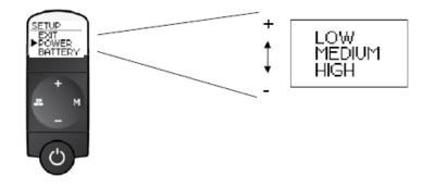
The power settings provide different degrees of power consumption. In general, the longer the stethoscope remains in an active mode, the greater its power consumption. The factory default is the LOW level. (NOTE: The Auto Off power management feature is further described below)
