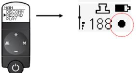
**3.** End the recording: Depress and release the (M) button. The stethoscope will stop recording and the recording icon will disappear from the LCD display. If the time between the beginning and ending of the recording session is greater than 29 seconds, only the last 29 seconds will be saved.
