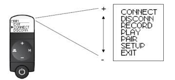
To leave the Main menu: Use the (M) button to select the "EXIT" option. This will return the stethoscope to its normal operating state.
