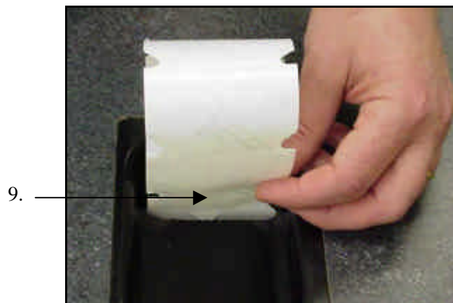
Figure 22: Pushing Leader Down into Slot of Feeder Opening
