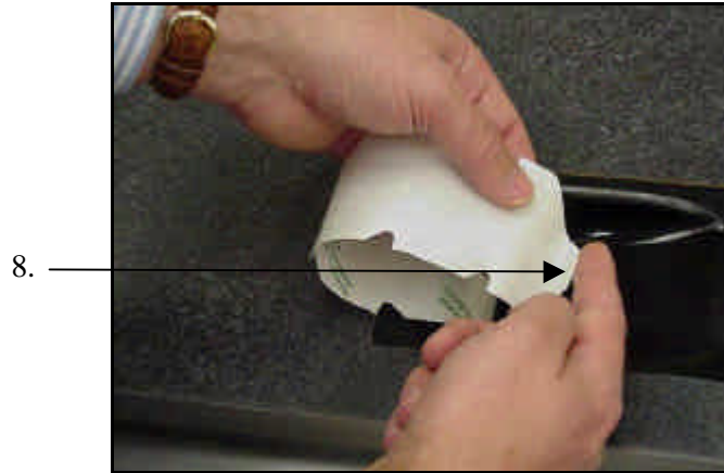
Figure 21: Putting a Slight Upward Bend in Leader
