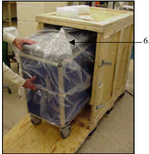
Figure 3: Removing Conversion Station and Backing Down Ramp
