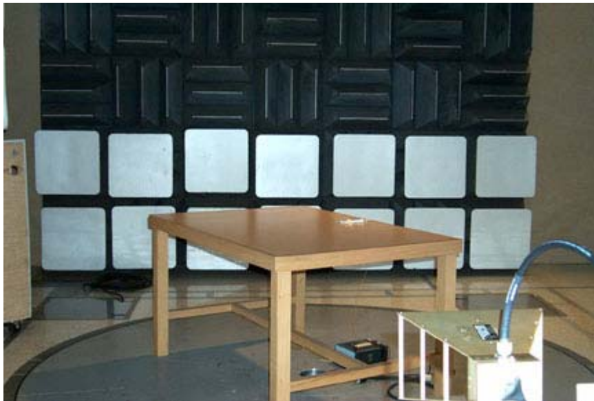
Transmitter Spurious and Radiated Emissions 1 to 5 GHz
