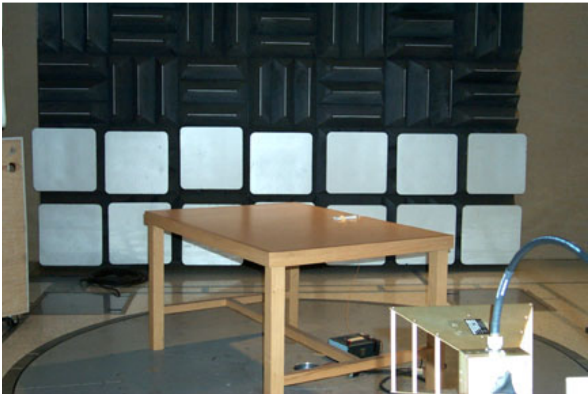
Conducted Emissions Test Setup (Remote)
