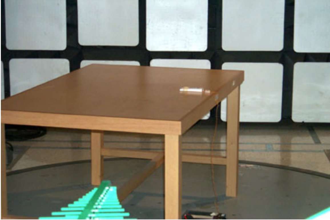
Radiated Emissions Test Setup (Remote)
