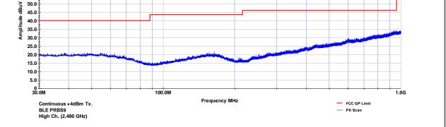
FCC Part 15.209 Radiated Emissions in restricted band - High Channel
