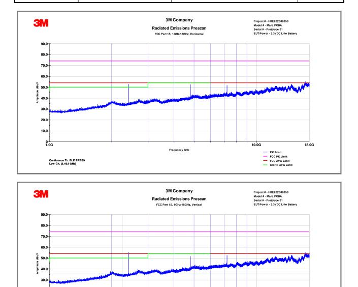
FCC Part 15.209 Radiated Emissions in restricted band - Low Channel
