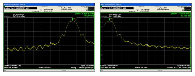
Band Edge - Low Channel Center Freq. 2.400GHz Band Edge - High Channel Center Freq. 2.4835GHz
