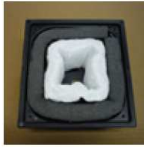
Fig.2 Install 3M foam and acoustic insulation.
