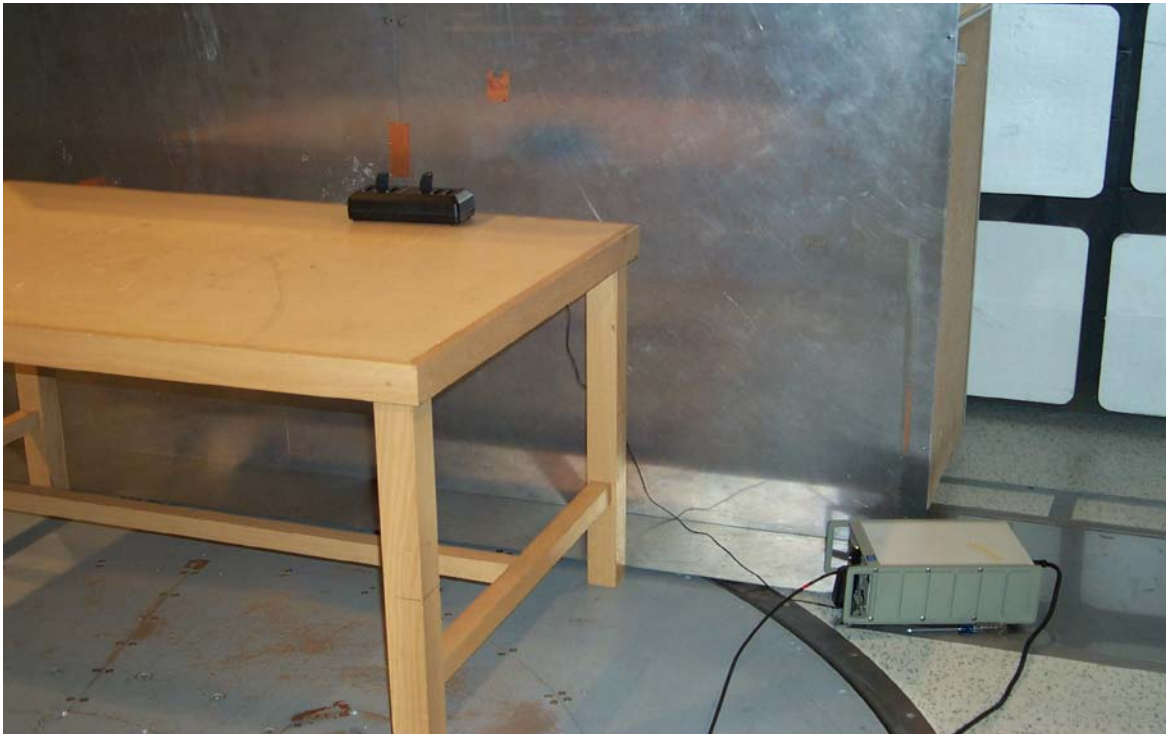
Conducted Emissions XT-1H Battery Charger
