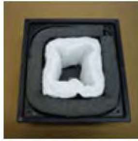
Fig.2 Install 3M foam and acoustic insulation.
