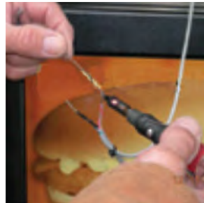
Fig.6 Solder all connections.
