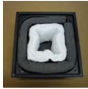
Fig.2 Install 3M foam and acoustic insulation.
