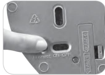
**(GB)** If the mouse and USB receiver do not connect, press the connect button on the USB receiver. The red LED indicator will blink slowly.
