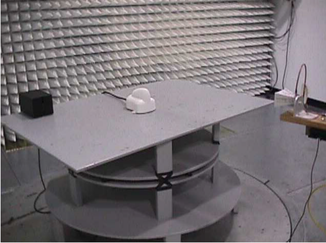
Radiated Emissions Test Configuration
