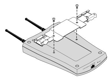
Align the T-rail grips with the ceiling T-rail, adjusting them so they grip the T-rail snugly. Tighten the screws on the T-rail grip. Position the antenna so that the arms point down and away from the access point at a 45° angle.
