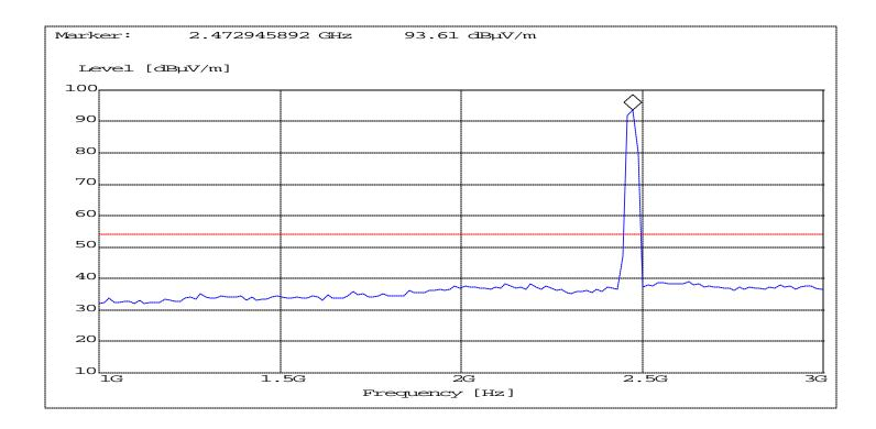
NOTE: The peak above the limit line is the carrier frequency.
