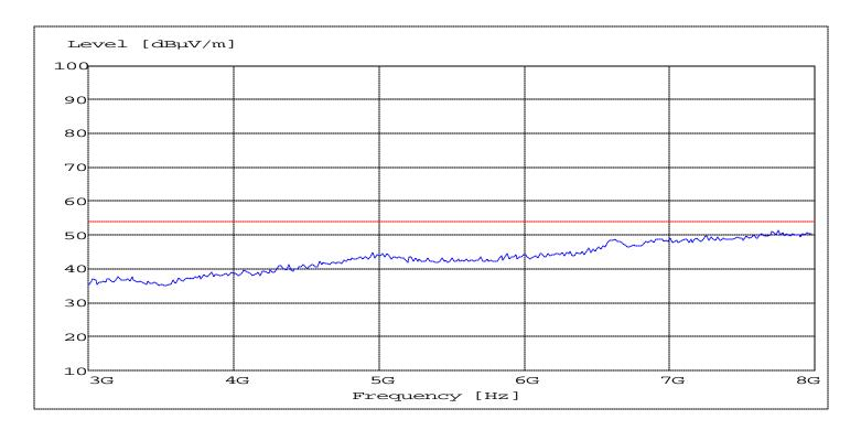
ANALYZER SETTINGS: f < 1 GHz: RBW/VBW: 100 kHz  $f^3 1 \text{GHz}$ : RBW/VBW: 1 MHz
