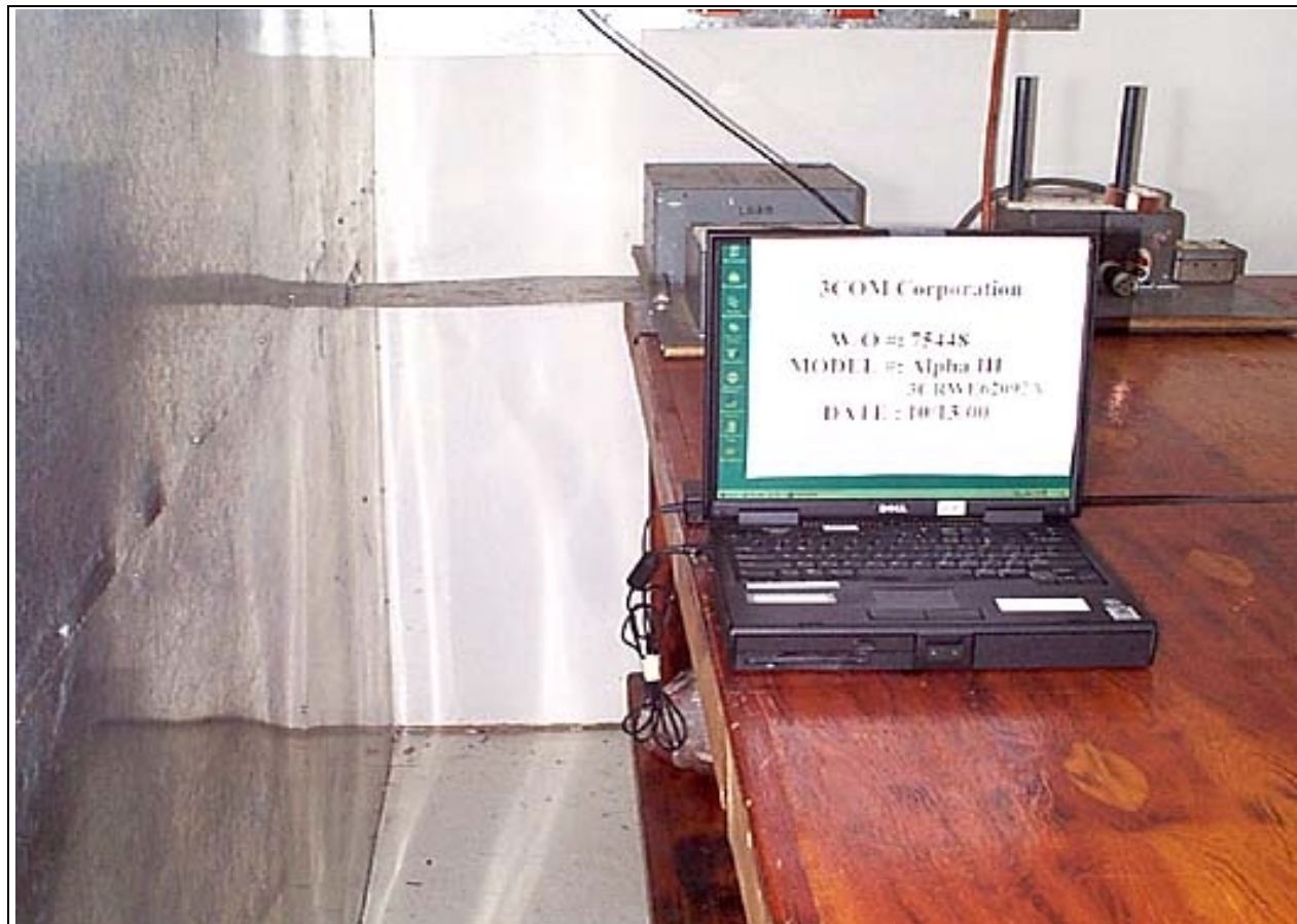
Conducted Emissions - Side View
