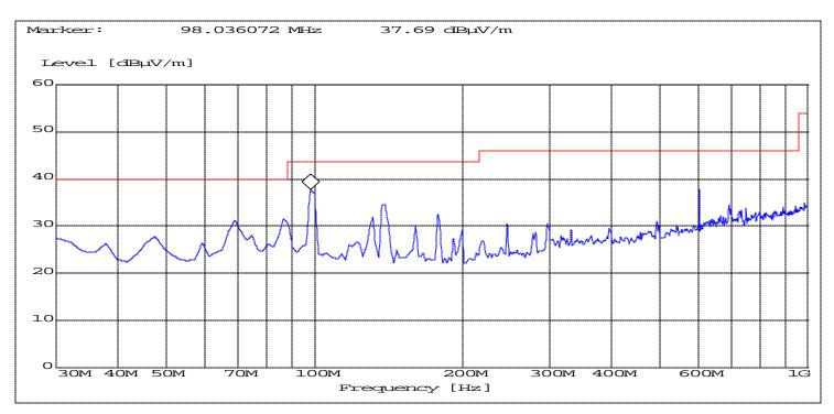
ANALYZER SETTINGS: f < 1 GHz: RBW/VBW: 100 kHz  $f^3$
