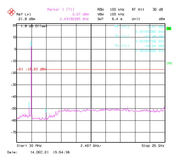
NOTE: The peak above the limit line is the carrier frequency.
