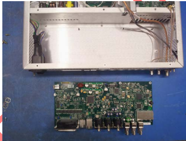
Figure 44 – Controller Exciter Outside Chassis
