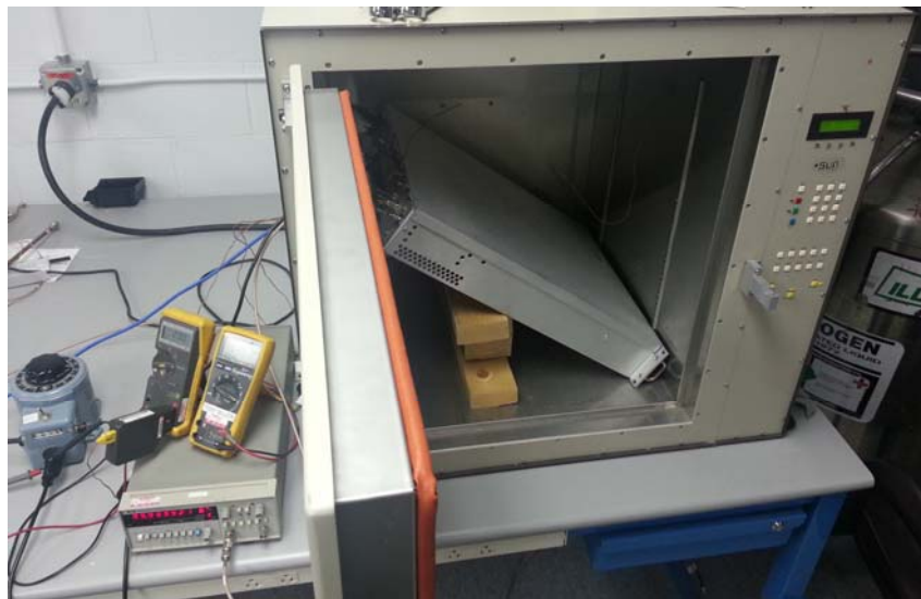
Figure 2: Setup for carrier frequency departure tolerance testing (shown with the door open to observe EUT positioning)
