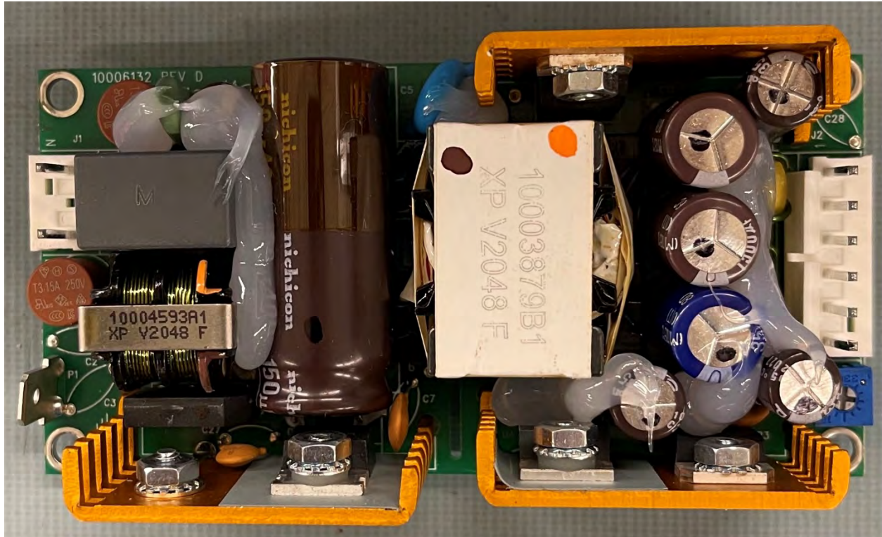
Controller Power Supply – Front View
