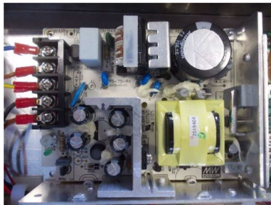
Fig. 11. Internal parts, close to view of AC/DC Switching Power supply.
