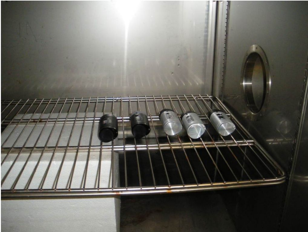
Test Setup for Frequency Stability Test
