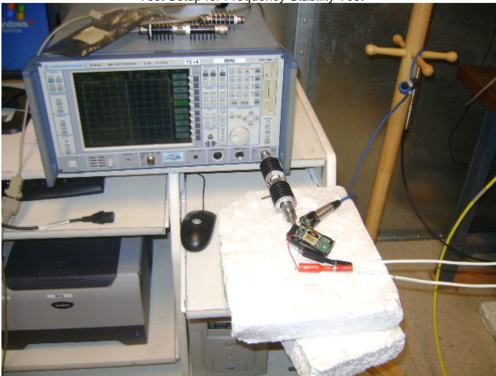
Test Setup for Occupied Bandwidth Test
