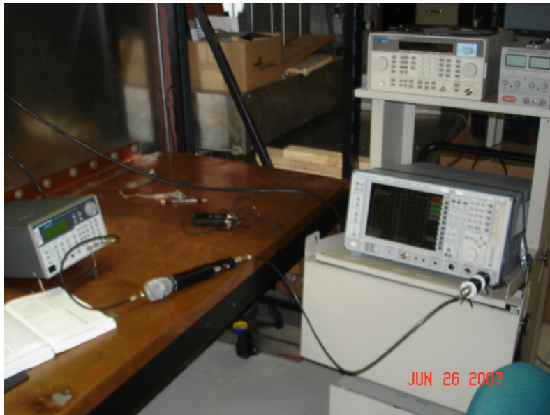
Occupied Bandwidth Test Set-up
