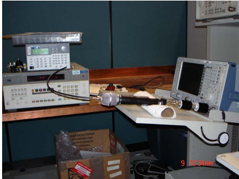
Antenna Conducted Emissions Test Set-up
