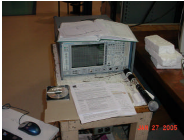
Output Power Test Setup
