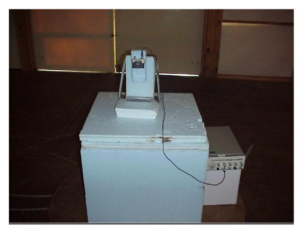
Photo Description: Radiated Spurious – Z Orientation
