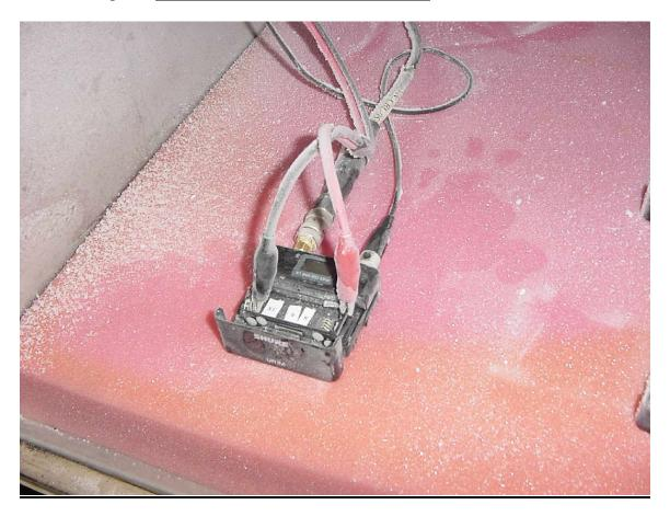
Photo Description: <u>Temperature Chamber – Frequency Stability</u>
