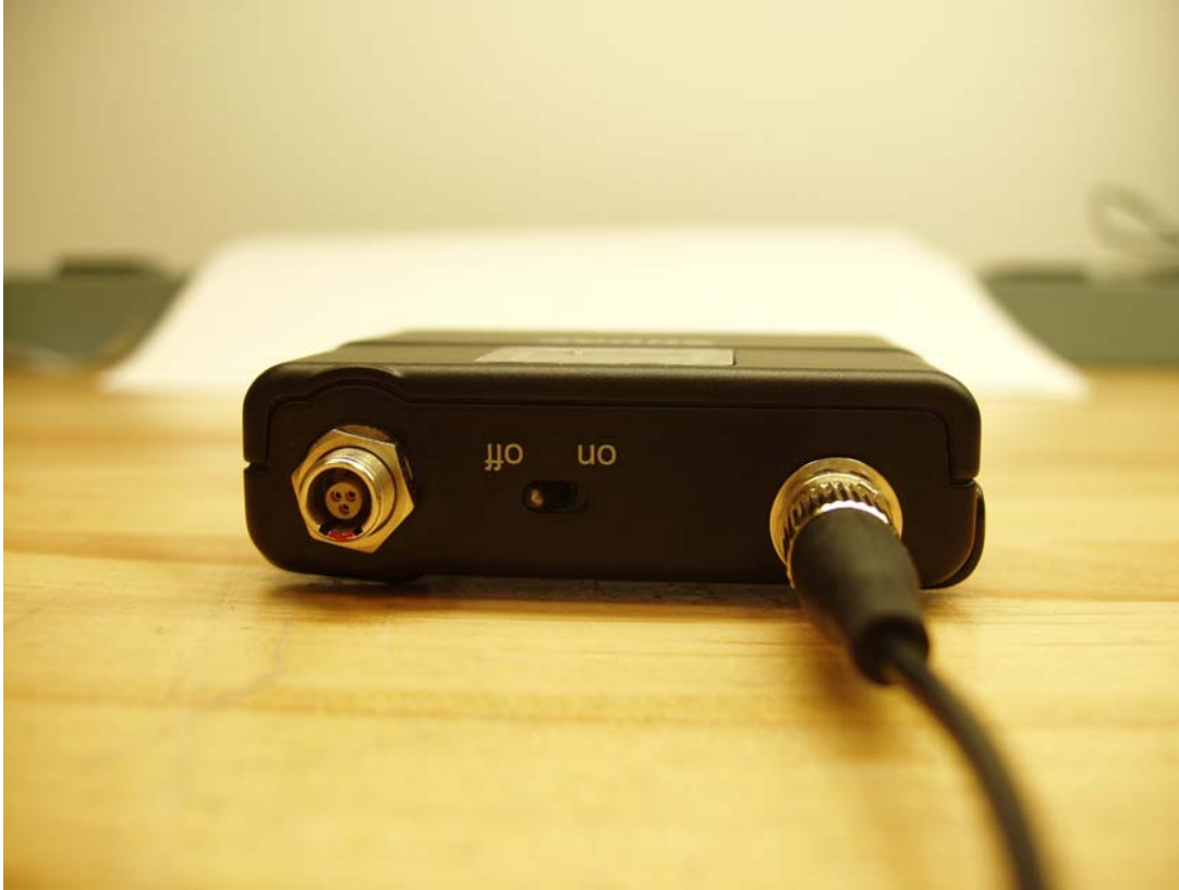
Shure UR1M Top View with LEMO3 Connector
