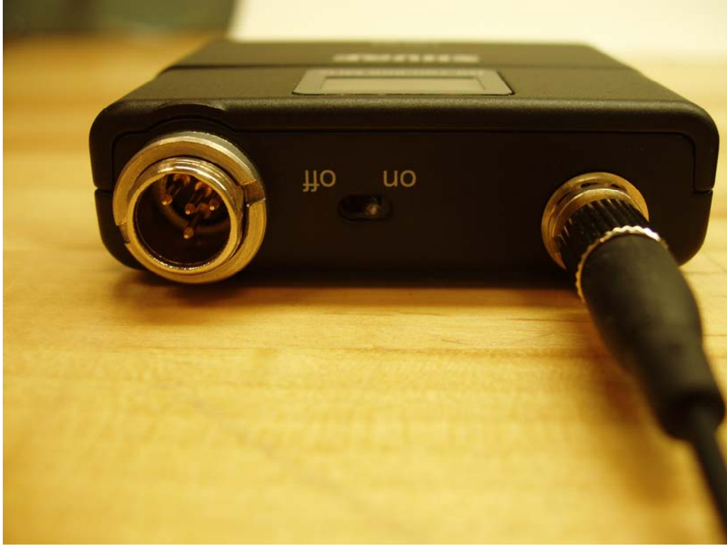
Shure UR1M Top View with TQG Connector
