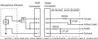
NOTE: LAVALIER MIC TIES PINS 3 AND 4 TOGETHER-GUITAR CABLE DOES NOT.
