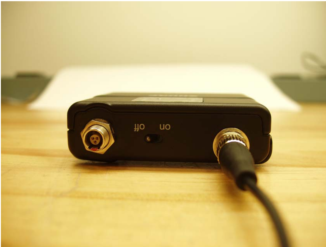
Shure UR1M Top View with LEMO3 Connector
