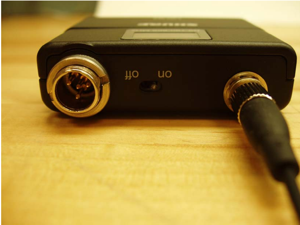
Shure UR1M Top View with TQG Connector
