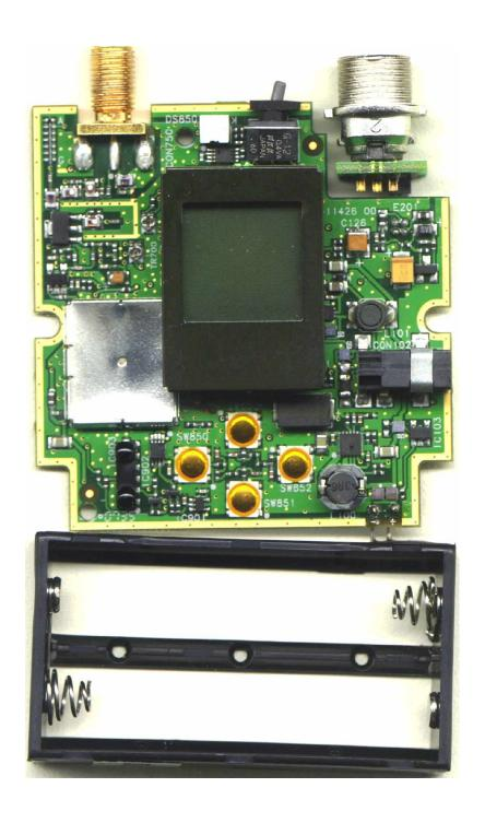
Photo Description: Front of circuit board with shield, display, and audio input board removed
