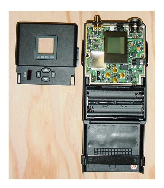
Photo Description: Circuit board removed
