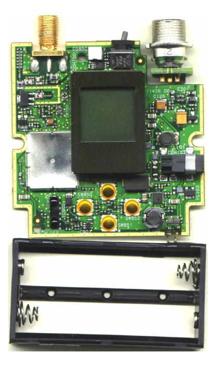
Company: Shure, Inc. Model: UR1H-H4 Date: 10-29-07 Photo Description: <u>Front of circuit board with shield, display, and audio input board removed</u>
