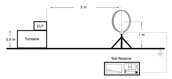
Below 1GHz Test Setup:
