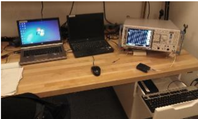
Figure B-1. Representative Test Setup for Frequency Stability
