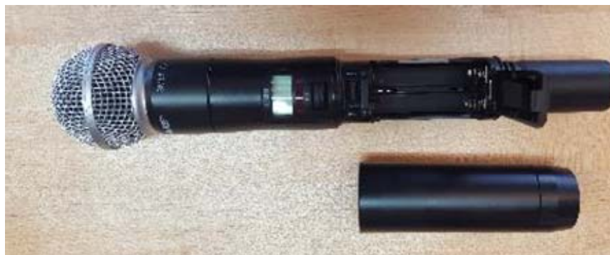
ULXD2 V50 Top, Battery Compartment Open
