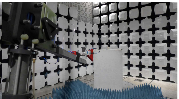
Figure 2: ULXD2 Transmitter Test Setup
