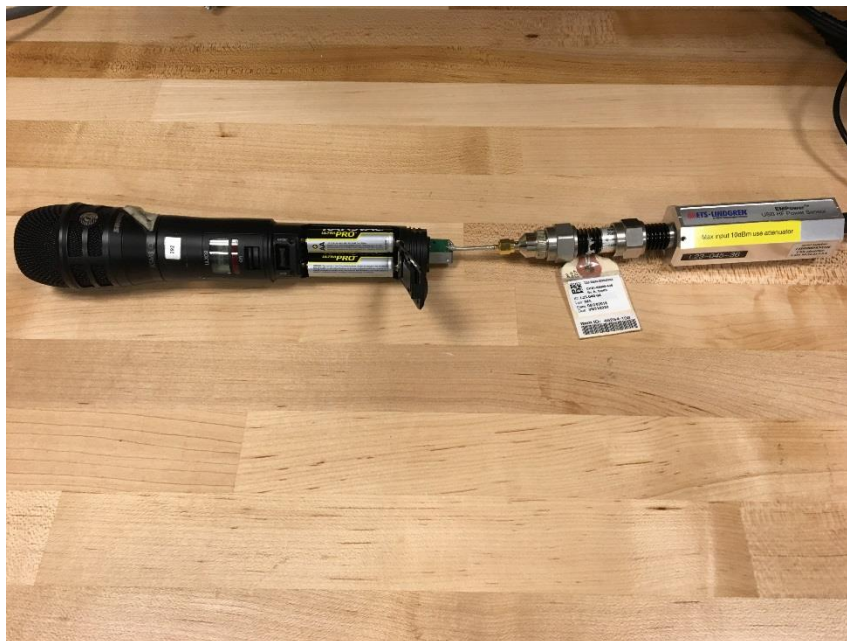
Figure B 1: Test setup for maximum peak conducted output
