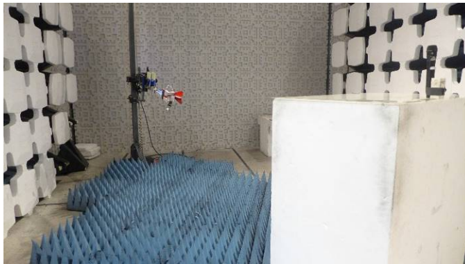
Test Setup for Unwanted Emissions and Field strength of fundamental
